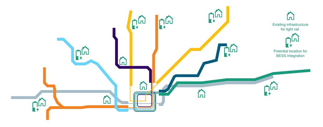
In addition to the energy exchange between vehicles, the recuperation of braking energy is possible in light rail networks with varying levels of potential. This requires the use of BESS.
